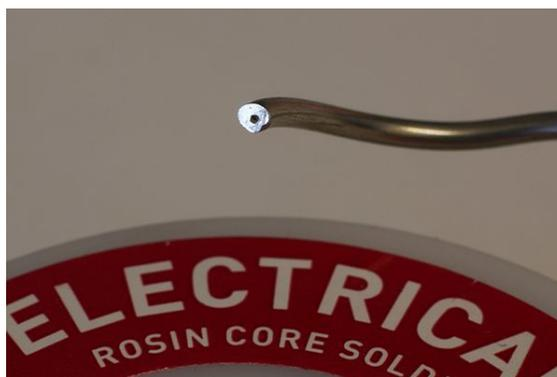
*Electrical solder with a rosin core, visible as a dark spot in the cut end of the solder wire.*
