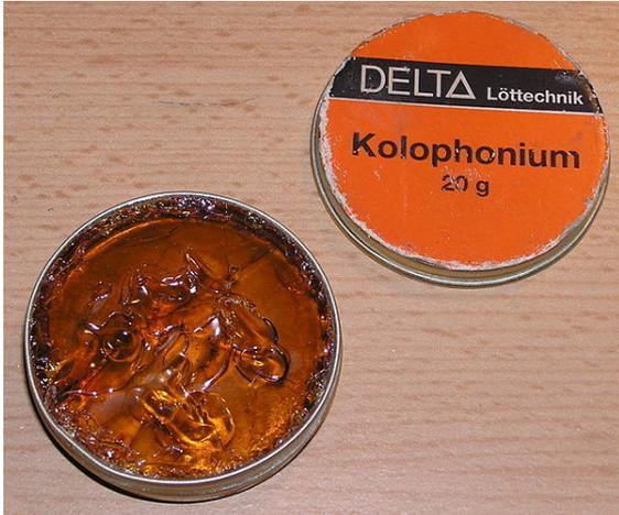
*Rosin used as flux for soldering*
