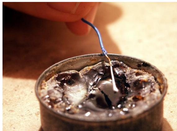
*Wire freshly coated with solder, still immersed in molten rosin flux*
